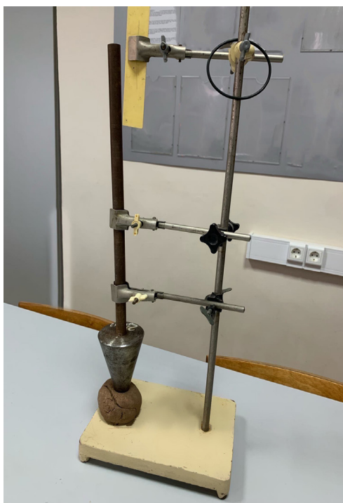
Fig. 4. Unit for determination the shear stress
